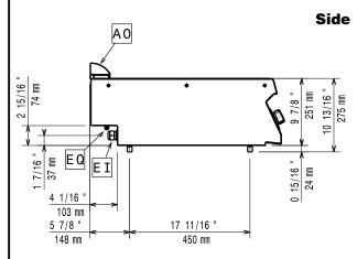
EI = Electrical connection EQ = Equipotential screw
