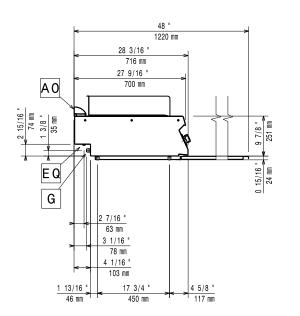
EQ = Equipotential screwF = Fumes outletG = Gas connection
