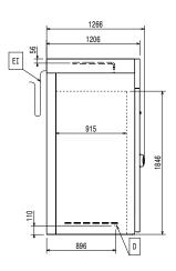
**EI** = Electrical inlet (power) Refrigerant Outlet
