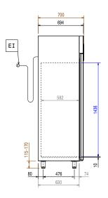
EI = Electrical inlet (power)RI = Refrigerant InletRO = Refrigerant Outlet
